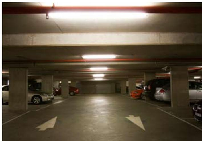
The Southbank Towers car park is significantly brighter and uses 25 per cent less energy since voltage reduction units and low mercury globes were installed
